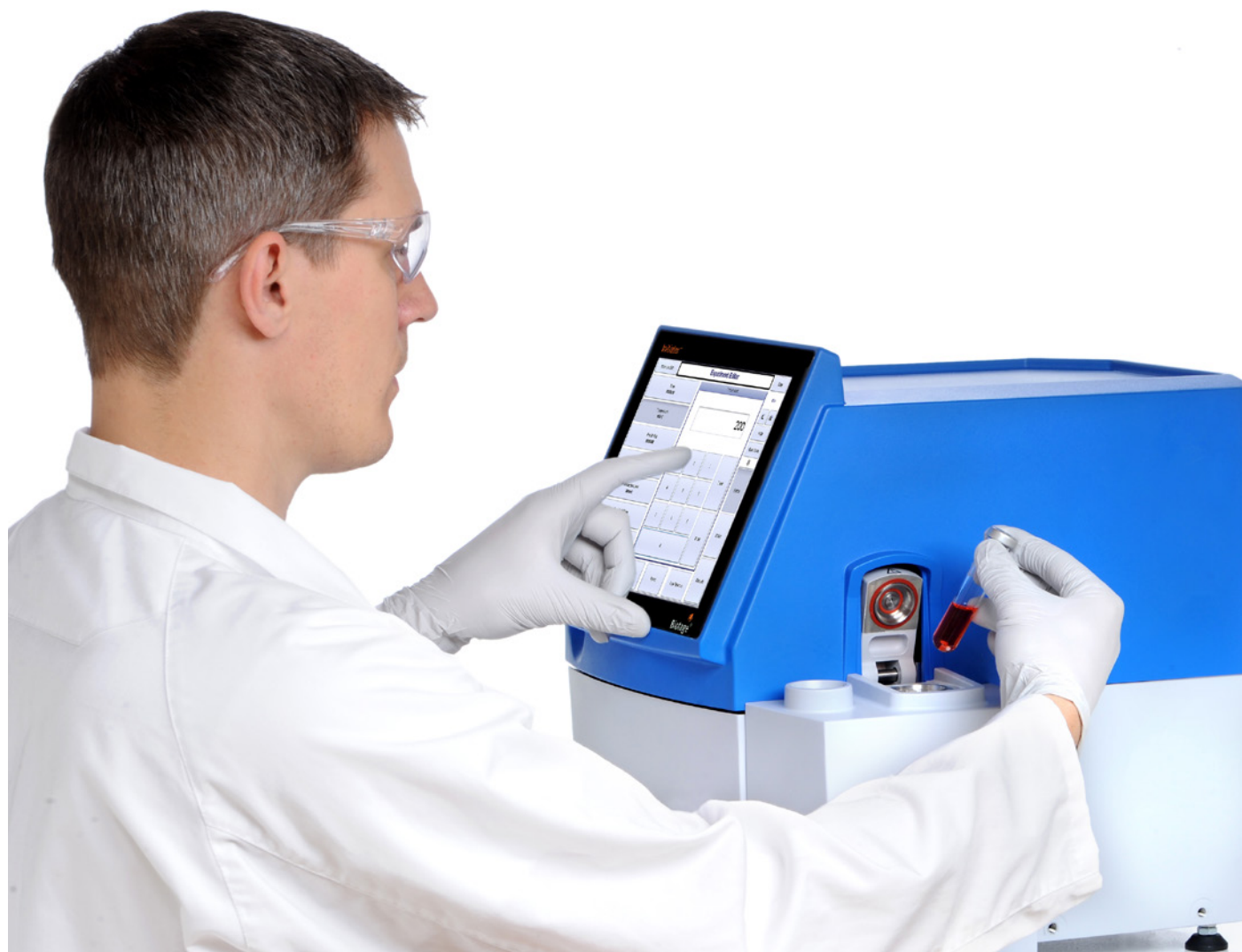
Figure 2. Biotage® Initiator+ is the standard tool for lab scale microwave assisted organic synthesis.
