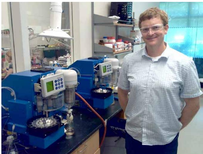
Biotage® V-10 is a key enabling tool at SBP, with its ability to rapidly remove solvent from the same scintillation vials used in the entire synthetic workflow. This application is so successful that the five chemists now keep two V-10s very busy.
